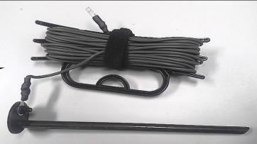
**Bushcomm single wire counterpoise** package designed for portable radio systems. Made with Kevlar cored PVC coated copper braid cable . Standard termination is with a flat blade terminal. Custom termination is available to suit your transceiver. Please call
