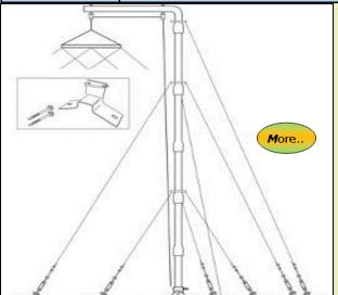
BU00648 - 10m tower with roof mounting kit, s/steel guys.. Ensure all safety measures and equipment are Back a page in place during erection.
