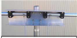
Leads showing the manner of attaching feedwires on the 5mm studs with wing nuts.
