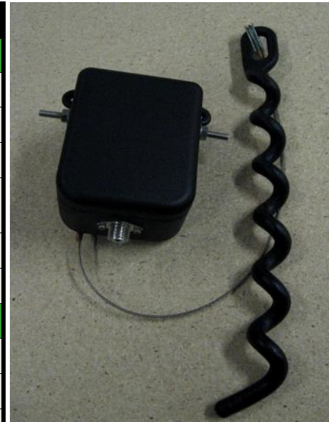
Above: Bushcomm Balun showing pigtail strain relief feature***
