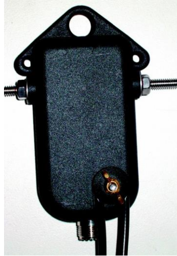
Left: Bushcomm Balun showing coaxial strain relief feature.****
