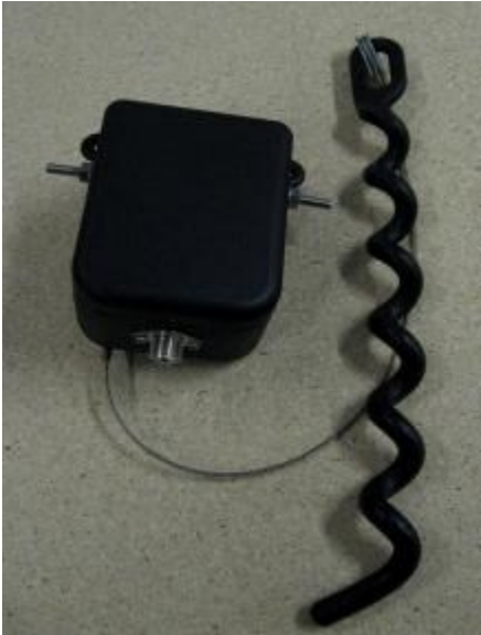
Above: Bushcomm Balun showing pigtail coax cable strain relief feature***
